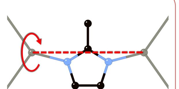
One of the Melm molecules is only connected to one Zn atom, so the framework is "interrupted". The channel system is not very open, and this is consistent with the the measured adsorption capacity. The structure of this new phase also nicely explains its good performance in the separation of CO<sub>2</sub> and CH<sub>4</sub>.
